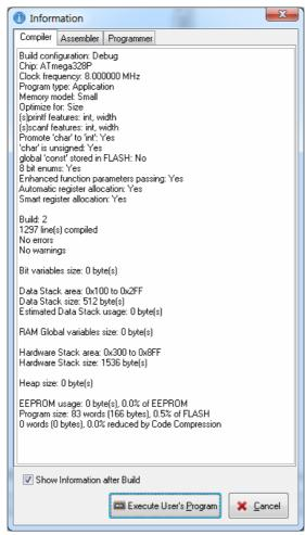
Press the **Execute User's Program** button to program the chip using the USBasp programmer.
